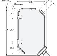
4.25 dia. vinyl-insulated round cable with 4conductors (Conductor cross section:0.3 mm², Insulator diameter: 1.05 mm), Standard length: 2 m
