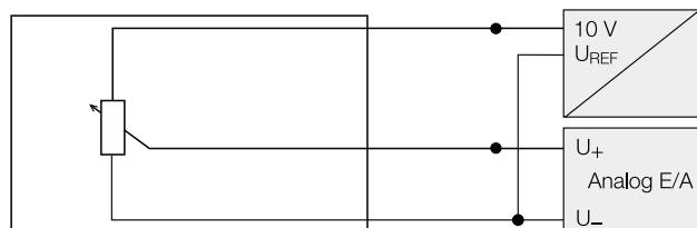
Connection scheme potentiometer, block diagram
