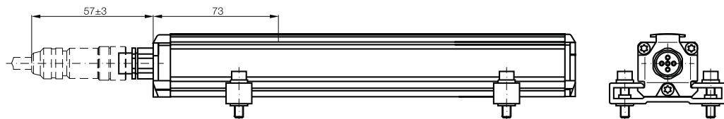
DeviceNet connection S93 with connector BKS-S92-00, BKS-S93-00 and BKS-S 48-15-CP-\_\_\_, page 254
