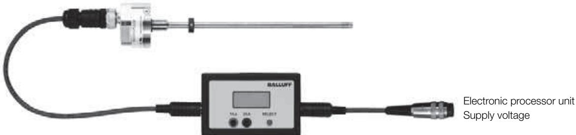
Set the output characteristic with the calibration box.
